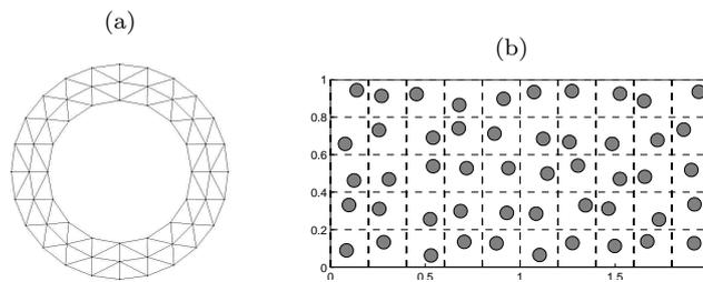
Figure 3. (a): reference mesh (b): random configuration of scatterers for  $\Phi = 0.1$
