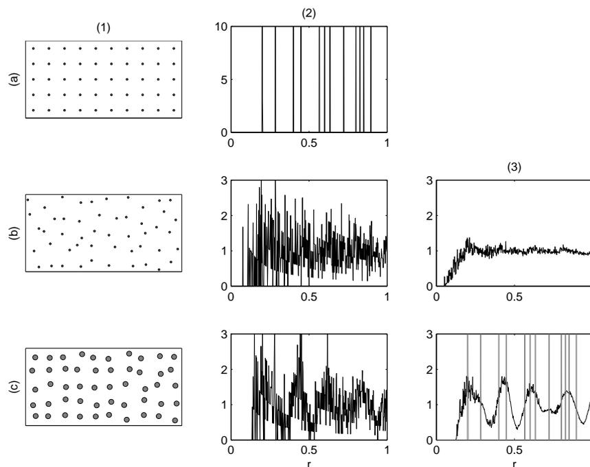
Figure 4. (a): periodic array; (b): perturbed square arrangement  $\Phi = 0.01$ ; (c):  $\Phi = 0.08$ ; (1): scatterers configurations; (2): RFD for one realization; (3): mean RFD for 500 realizations
