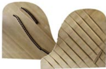
Figure 3: Soundboard with briges (left) and ribs (right).
