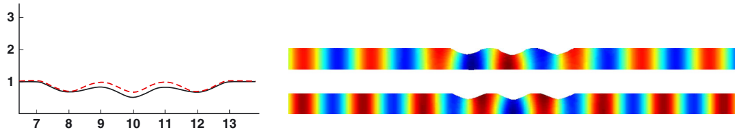
Figure 10. Left: initial cavity in continuous line, final cavity in dashed line, for \varepsilon = .5 , Right: Re(u) for the invisible deformation at the two frequencies k_1 and k_2 .
