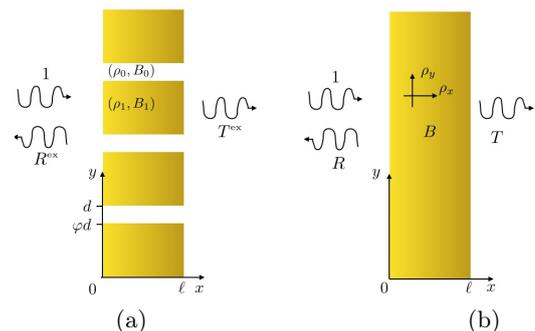
FIG. 1: (a) Geometry of the array. (b) Equivalent birefringent layer.
