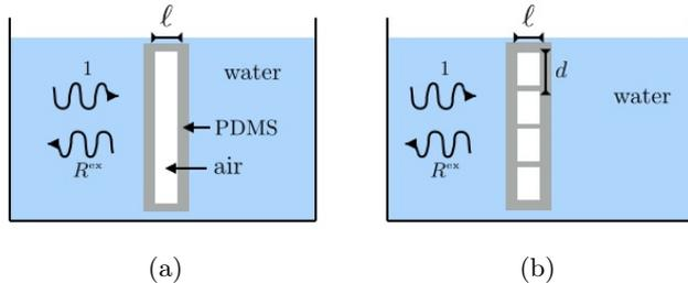
FIG. 4: Example of possible set-up. (a) Guided waves by a layer of air in water ( $\varphi = 1$ ). (b) Spoofer plasmon in a structured array of air inclusions in water. In practice, air can be encapsulated in PDMS;  $d = 0.5$  mm and  $\ell = 0.1d$  or  $\ell = d$ .
